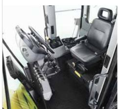
he RG200.B grader has various features to improve operator comfort: adjustable seat with armrest and headrest and elastic suspension, adjustable for the weight of the operator.
